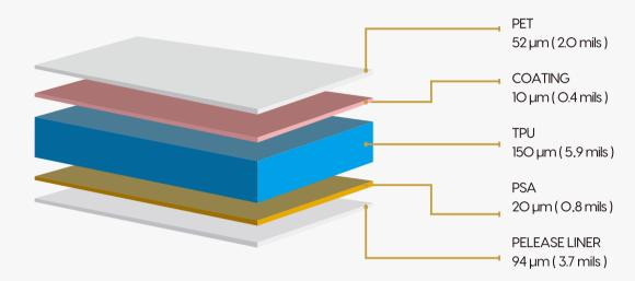
OVERALL THICKNESS 180 µm (7.1mils)+/- 5%
