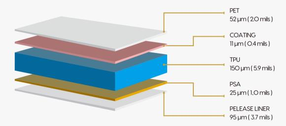
OVERALL THICKNESS 186 µm (7.3mils)+/- 5%
