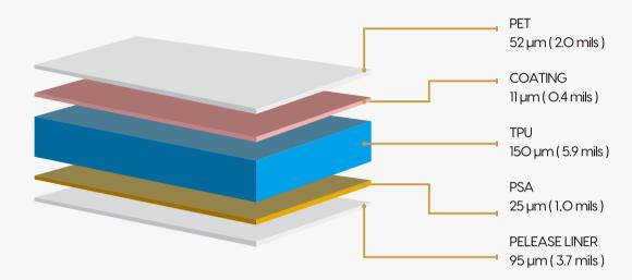
OVERALL THICKNESS 186 µm (7.3mils)+/- 5%
